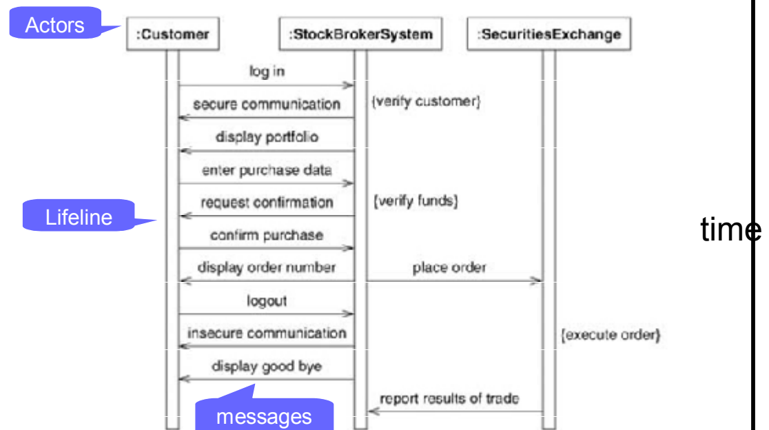
Figure 7.5 Sequence diagram for a session with an online stock broker. A sequence diagram shows the participants in an interaction and the sequence of messages among them.
