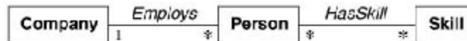
Figure 15.5 Analysis model for person skills. Derived data is undesirable during analysis because it does not add information.
