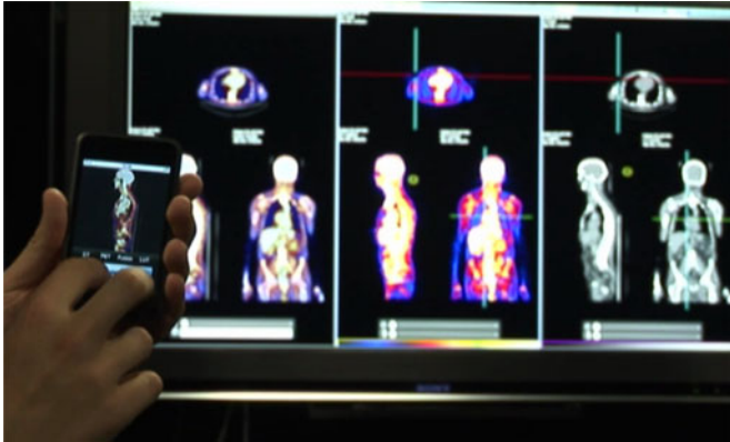
Fig. 6. SparkMed in use synchronizing a handheld visualization system (shown being manipulated by hand on the left of the image) with the hospital's corresponding data source (shown on the screen in the background).
