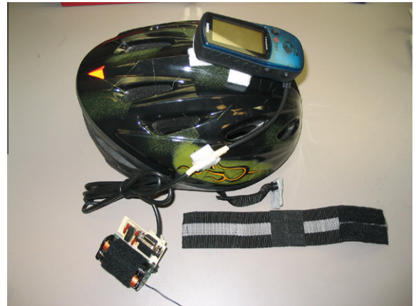
Fig. 3. Master node assembly.
